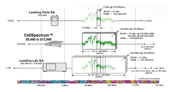
Whether in the lab, facility, field or across the city, **CellSpectrum™** is the only platform that enables universal spectrum analysis and RF path characterization for all wireless communications. It is a unique product in the market and a must have solution for the wireless industry.
